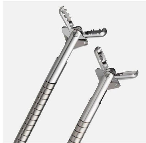
Figure 3: SpyBite™ (right) and SpyBite Max™ (left) biopsy forceps. The SpyBite Max forceps is 286 cm long, 1 mm in diameter, jaw opening of 4.1 mm, and has serrated teeth and elongated fenestration holes in the biopsy cups to acquire larger tissue specimens.
