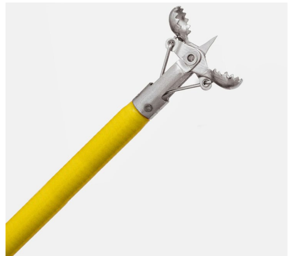
Figure 1: A double-bite forceps with a needle spike between opposing biopsy cups. This forceps allows the acquisition of two biopsy pieces per forceps passes. The first biopsy specimen is secured on the needle spike during the collection of the second specimen.
